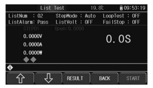
Note: enter test page to start test, the page displays the test and compare result of current test step.
