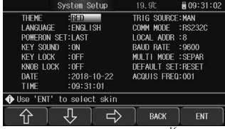
On the page, the system style and application can be set, press [Ent] to switch the menu, input umber to set date and time then press [Ent] to confirm
