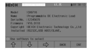
Display the full system information and installed module of the tester, any change is unavailable
