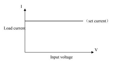
Press **(**CC**)** to enter CC mode, the key is light, input the current value, and the number is displayed in status bar **IS = 0.0000A**
